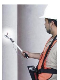
Accurately pinpoints steel reinforcing bars, or "rebars" in concrete; (typically 8-9" depth for 1/2" diameter rebar)
