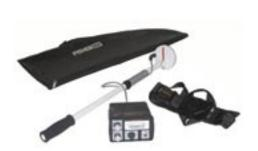
The Fisher M-101 metal detector was designed specifically for finding reinforcing bars and other metal objects embedded in concrete, conduits, PK nails, wiring, wall studs and other metallic objects. Users may expect accuracy to 1/4" of the centerline of the rebar.
